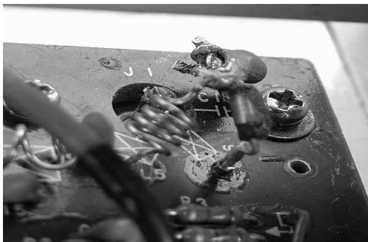
Figure 4: FT271 PA unit, antenna connector J1
